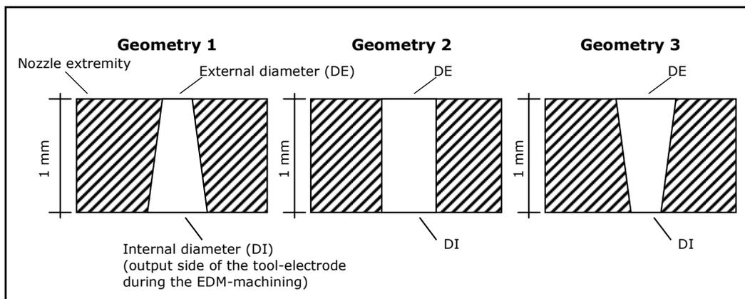
**Fig. 3:** Possible geometries of microholes in the injection nozzle according to an adjustment of Com and Gain
