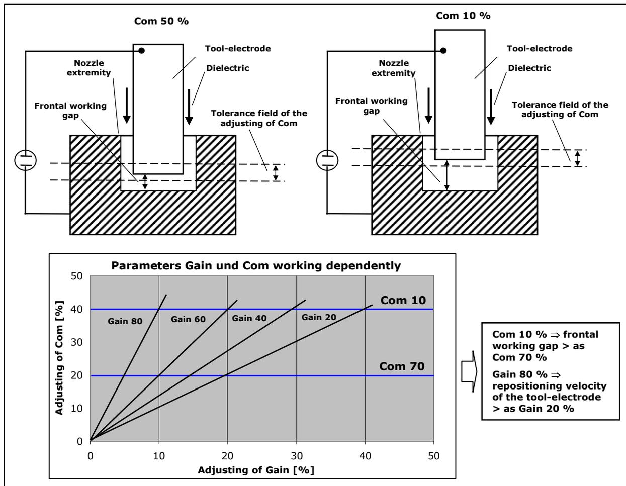
**Figure 4:** Operation principle of Com and Gain of the closed-loop control of the EDM-machine AGIE Quadraton I
