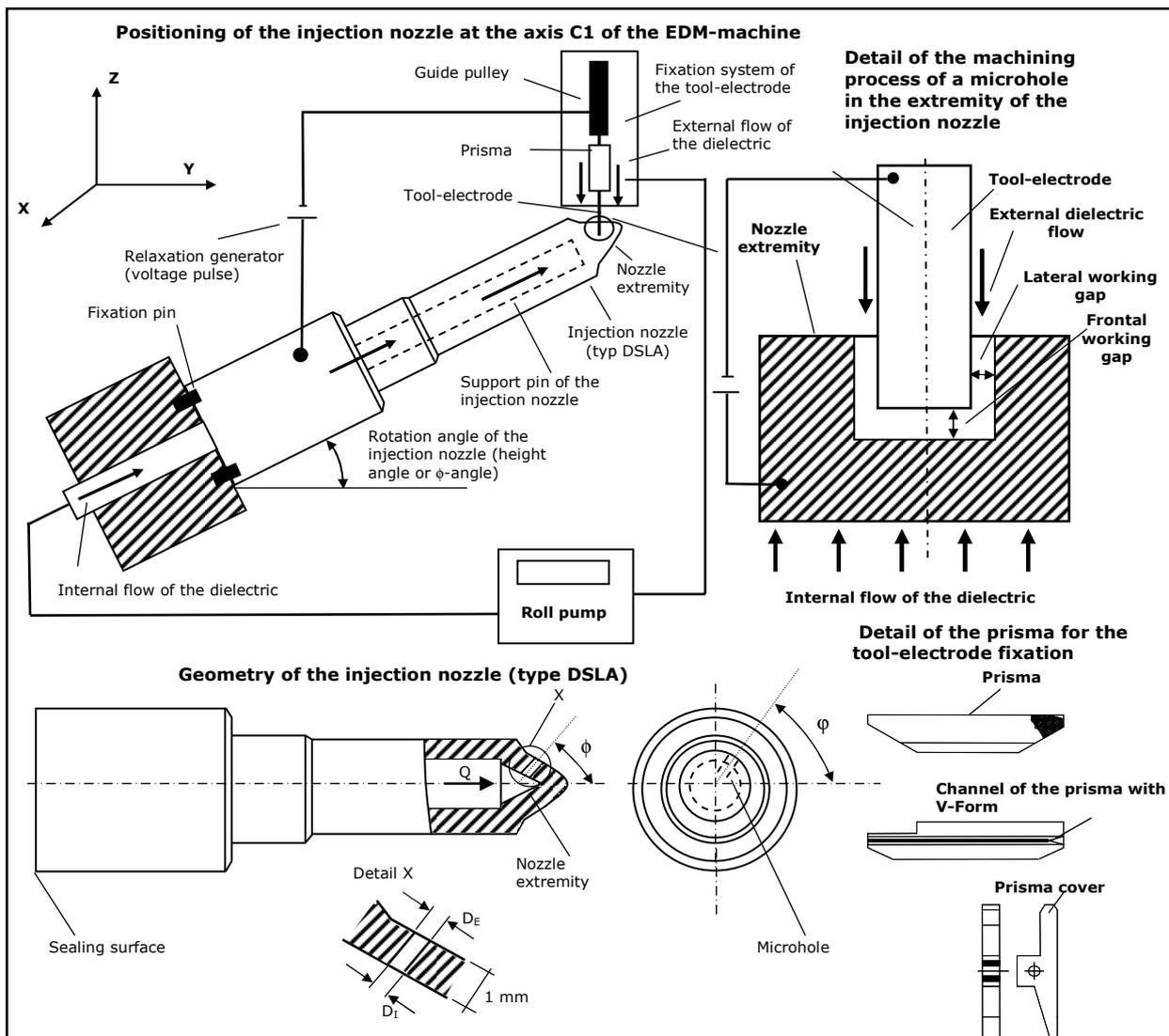
**Fig.2:** Positioning of the injection nozzle (workpiece) at the axis C1
