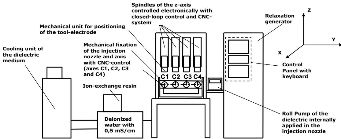
**Fig.1:** Main technological characteristics of the machine AGIE Quadraton I used in the experiments
