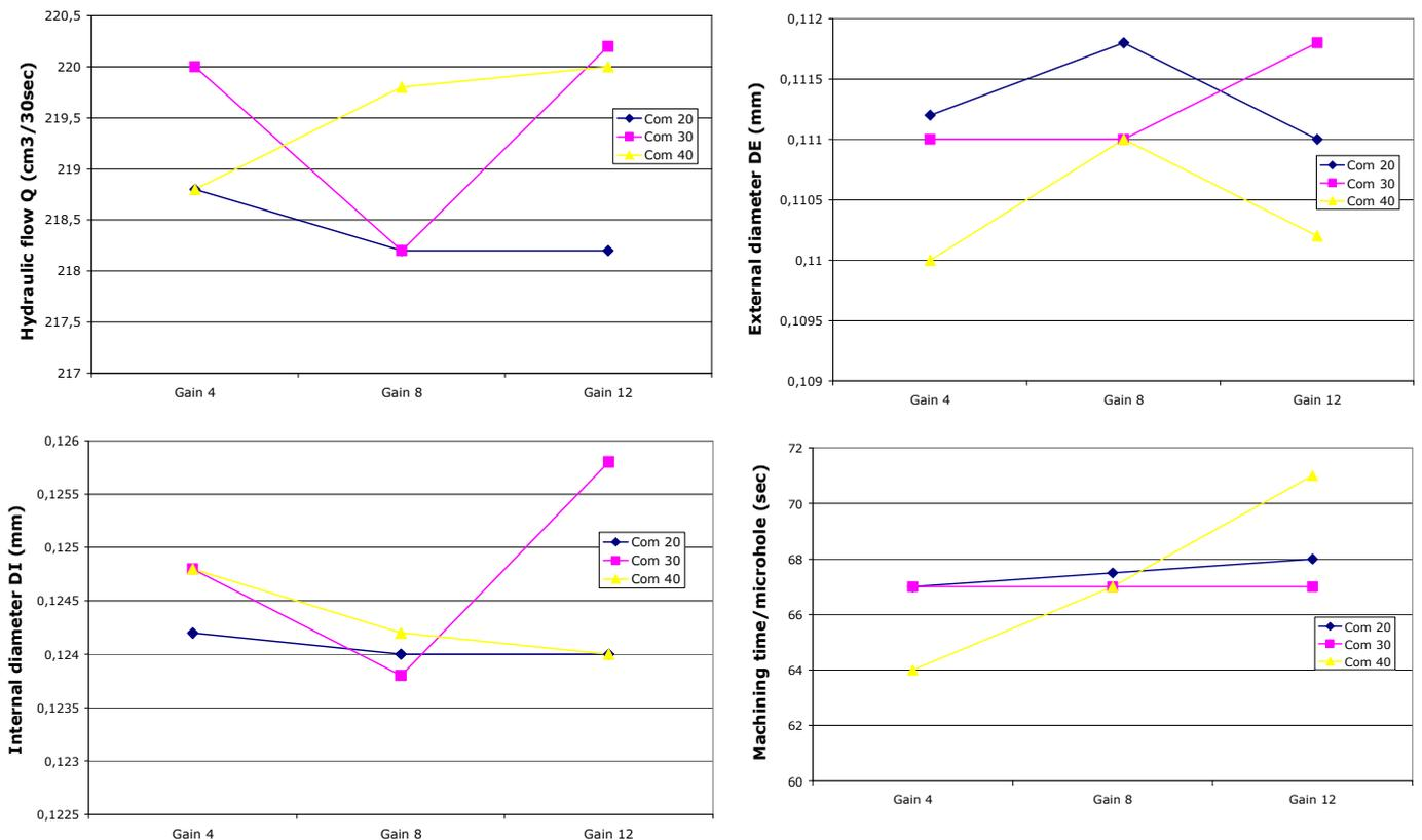
**Figure 3-A:** Experimental results related to the machining depth 3
