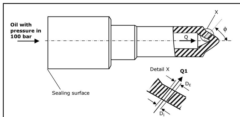
**Fig. 3:** Measuring procedure of the hydraulic flow of an injection nozzle after the machining process
