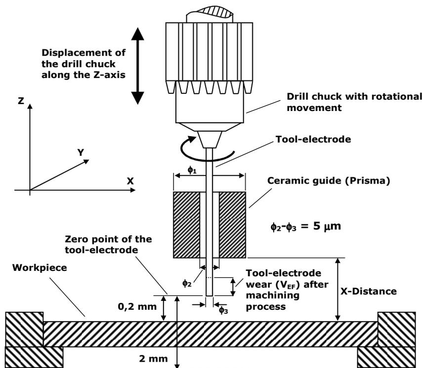
Figure 4: Assembling details of the ceramic guide of the tool-electrode in the Z-axis of the machine
