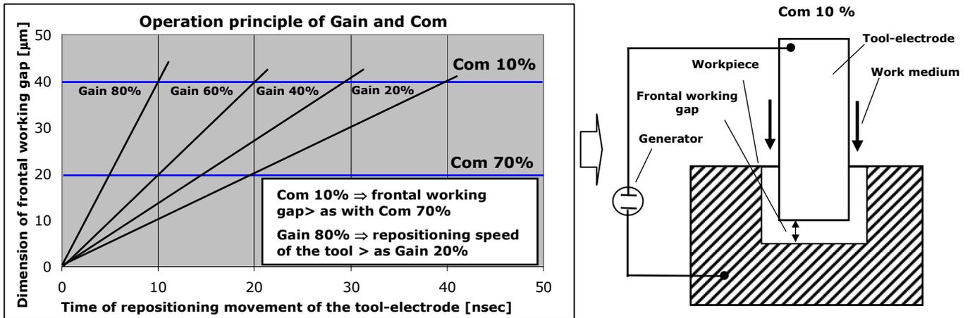
Figure 3: Interaction of Com and Gain of the closed-loop control system (AGIE Compact 1)
