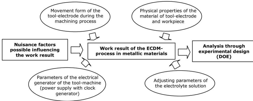
**Figure 1:** Parameters of the ECDM-technology influencing the work result of the machining process (input-variables to be modified in experiments)
