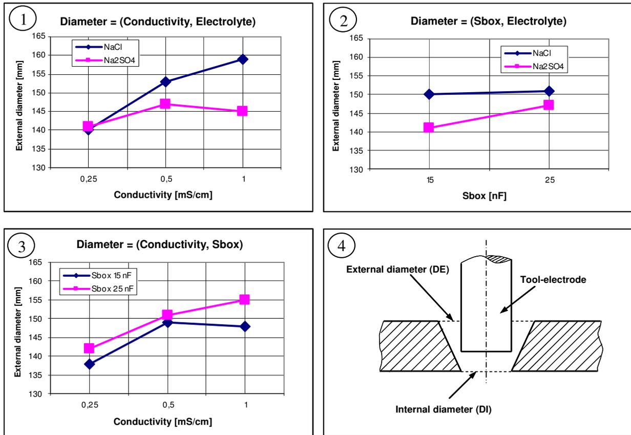
**Figure 11:** Influence of ECDM-parameters on the external diameter of the microhole
