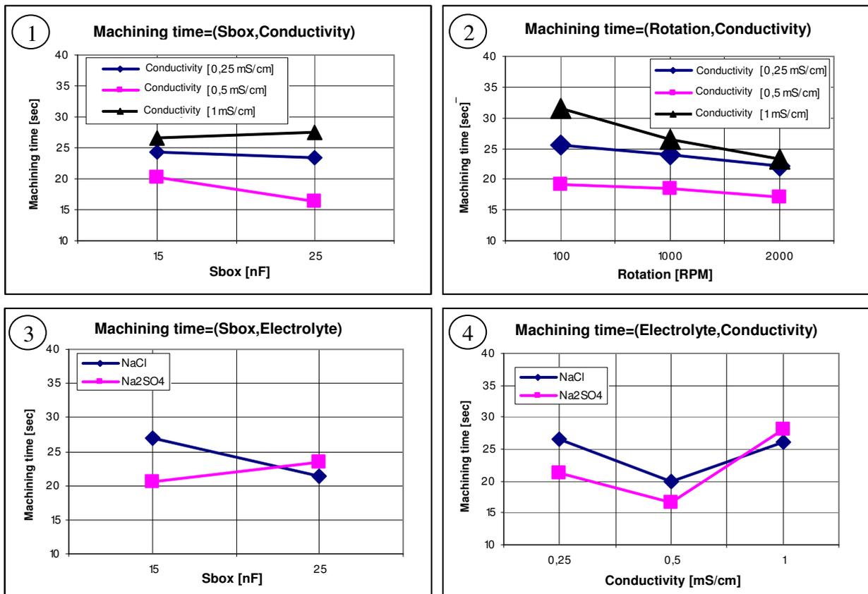
Figure 6: Result related to the machining time of the ECDM-process
