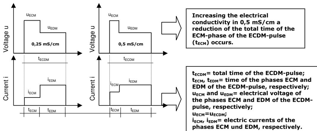
Figure 7: Influence of the electrical conductivity on the characteristics of the ECDM-Pulse
