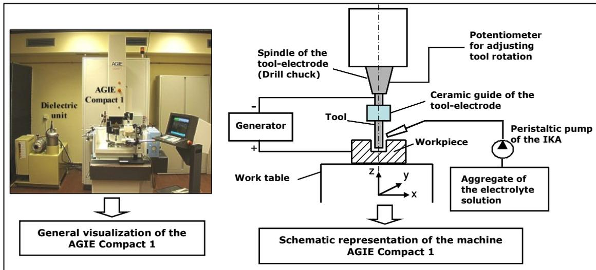
Figure 2: AGIE Compact 1 applied in the experimental investigations of the ECDM-technology
