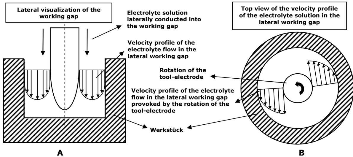
**Figure 8:** Velocity profile of the electrolyte flow in the working gap provoked by the rotation of the tool-electrode
