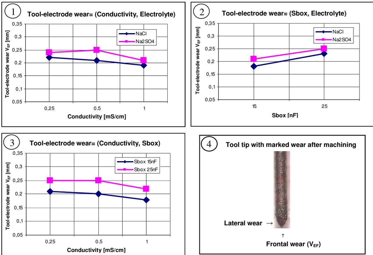
Figure 10: Influence of the modification of ECDM-parameters on the tool-electrode wear
