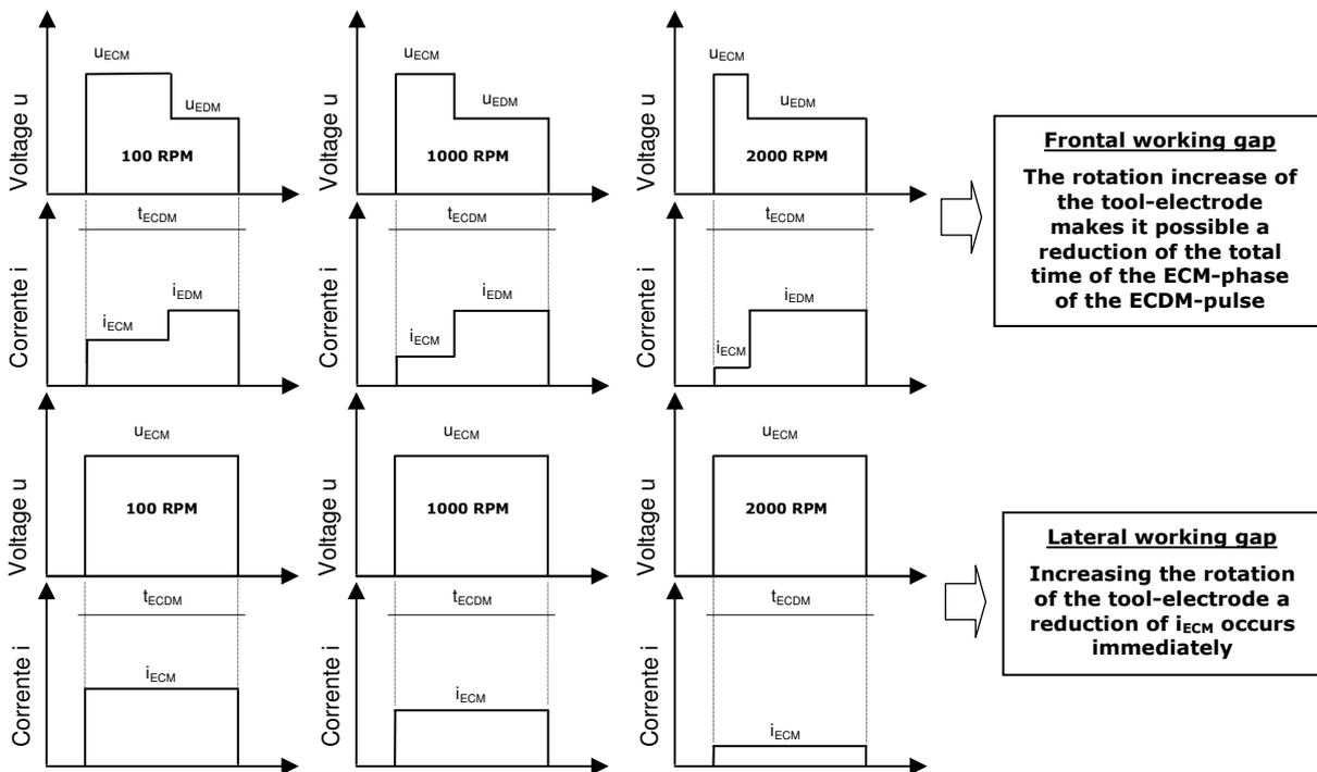
**Figure 9:** Influence of the tool-electrode rotation on the output variable of the ECDM-pulse
