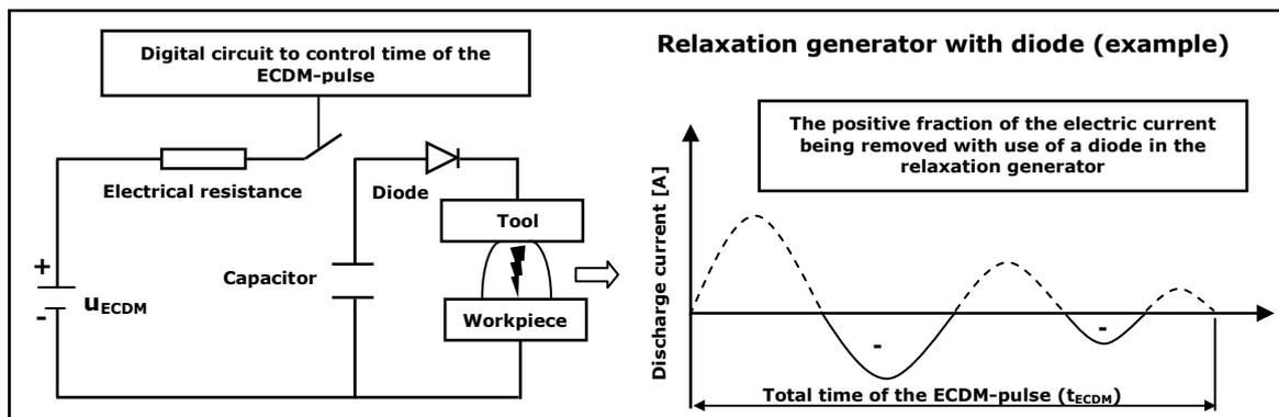
**Figure 5:** Basic operating principle of the parameter *Sbox* in the generator of the AGIE Compact 1
