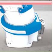
FULL - COLLABORATIVE SPEED SWITCH (Controller option + Safety device installed)
