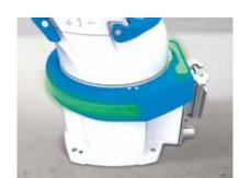
**BLUE:** manual restart after collision Blinking BLUE: automatic restart after collision.
